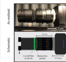
"Researchers have developed a metasurface attachment that can turn just about any camera or imaging system, even off-the-shelf systems, into polarization cameras. The attachment uses a metasurface of subwavelength nanopillars to direct light based on its polarization and compiles an image that captures polarization at every pixel."
