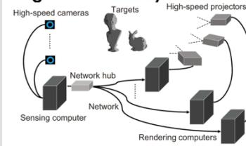
"A challenge to adopting augmented reality (AR) in wider applications is working with dynamic objects, owing to a delay between their movement and the projection of light onto their new position. But, Tokyo Tech scientists may have a workaround. They have developed a method that uses multiple projectors while reducing delay time."
