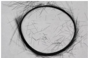
"Researchers have developed a way to make lightweight fibers, for possible use in the bodies of cars, out of an ultracheap feedstock: the waste material from the refining of petroleum."
