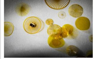
"Inspired by how dandelions use the wind to distribute their seeds, a team has developed a tiny sensor-carrying device that can be blown by the wind as it tumbles toward the ground."
