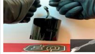
"Researchers have created A material that is very stretchable and extremely tough. The material is of A type of ionogel, which is polymer network that contain salts that are liquid at room temperature. The new material has the stretchability of polyacrylic acid and is stronger than polyacrylamide. In terms of toughness, it's better than cartilage."
