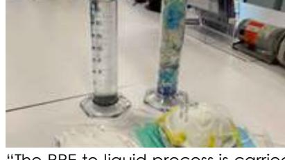
"The PPE-to-liquid process is carried out at a temperature of 300°C and takes about an hour in a small prototype machine in a laboratory in the faculty. Gaseous by-products from the process are oxygen and low concentrations of carbon dioxide which can be safely discharged."
