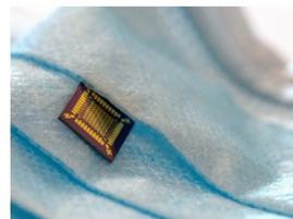
"Silk woven into transistors can result in highly sensitive, ultra-fast sensors, new findings that could open doors to many other applications for the hybrid devices.
