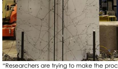
"Researchers are trying to make the process more efficient and definitive by using artificial intelligence, combined with a classic mathematical method for quantifying web-like networks, to determine how damaged a concrete structure is, based solely on its pattern of cracking. Read more in this [paper](#)."
