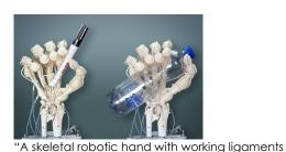
and tendons can now be 3D-printed in one run. The creepy accomplishment was made possible by a new approach to additive manufacturing that can print both rigid and elastic materials at the same time in high resolution.
