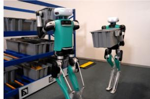
"Agility Robotics has taken the wraps off its next-gen bipedal bot, which comes with some noticeable upgrades — namely, a cylindrical head and two animated LED "eyes." In a press release, the company says it made the changes to its warehouse-friendly bot, called Digit, to improve "human robot interaction."
