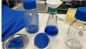
"In a new study, North Carolina State University researchers found they could separate blended cotton and polyester fabric using enzymes — nature's tools for speeding chemical reactions. Ultimately, they hope their findings will lead to a more efficient way to recycle the fabric's component materials, thereby reducing textile waste."
