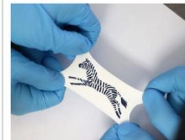
"Researchers have now made a thermoelectric generator (TEG) that is soft and stretchy and that biodegrades completely when exposed to the environment. Unlike conventional rigid thermoelectric devices, this one, reported in the journal Science Advances, could be easily integrated into fabrics, allowing for body-heat-powered wearable sensors or temperature-detecting disposable face masks."
