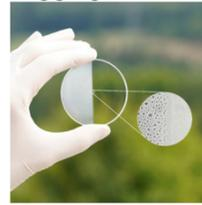
"Researchers have developed an optical coating system that combines antifogging and antireflective properties. The new technology could help boost the performance of lidar systems and cameras."
