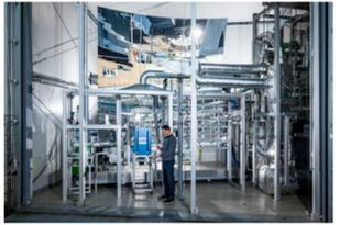
"In the first project phase, the research team constructed a container-sized test facility, which now went into operation. This first-phase installation removes two kilograms of CO2 from the ambient air in one day and turns it into 0.5 kilogram of solid carbon."
