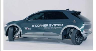
"Car manufacturer Hyundai has revealed an Ioniq 5 car with wheels that can rotate up to 90 degrees so that it can "crab" drive sideways at this year's Consumer Electronics Show.
