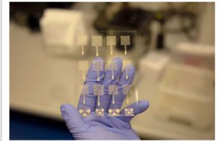
"The study, led by Washington State University researchers, demonstrates that electrodes can be made using just screen printing, creating a stretchable, durable circuit pattern that can be transferred to fabric and worn directly on human skin. Such wearable electronics can be used for health monitoring in hospitals or at home."
