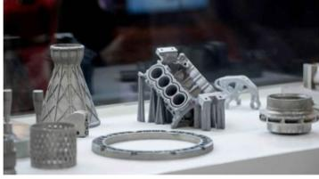
"Many industries rely on metal additive manufacturing to rapidly build parts and components. Rocket engine nozzles, pistons for high performance cars, and custom orthopedic implants are all made using additive manufacturing, a process that involves building parts layer-by-layer using a 3D printer."
