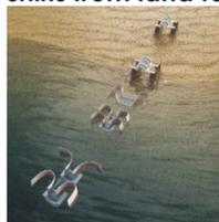
"The bistable actuator is made of 3D-printed soft rubber containing shape-memory alloy springs that react to electrical currents by contracting, which causes the actuator to bend. The team used this bistable motion to change the actuator or robot's shape. Once the robot changes shape, it is stable until another electrical charge morphs it back to its previous configuration."
