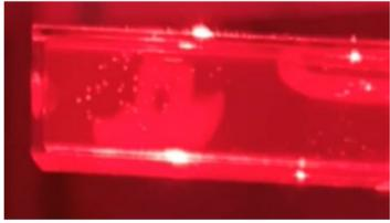
"Researchers describe a technique of volumetric 3D printing that goes beyond the bottom-up, layered approach. The process eliminates the need for support structures because the resin it creates is self-supporting."
