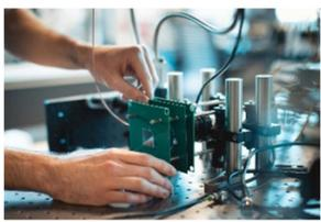
"Now researchers at Stanford University have developed an innovative system that can integrate with almost any mass-produced CMOS image sensor to capture 3D data at potentially a fraction of the price of today's lidars. It relies on the piezoelectric effect, the process by which deforming some materials generates electricity, and vice versa."
