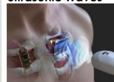
"Ultrasonic waves have applications in wireless charging of batteries underwater or in body-implanted electronic devices."
