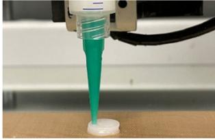
"For the purpose of personalised therapies, the UPV/EHU's 'Materials+Technologies' (GMT) Group has used 3D printing to develop tablets based on different types of starch, and has confirmed that drug release could be tailored by optimising the right starch type and tablet shape."
