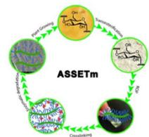
"Soft, wearable sensors can improve our lives, but these soft and stretchable electronic devices are nearly impossible to recycle. As a result, this electronic waste usually ends up in landfills or polluting the environment. Polymer scientists from the University of Groningen have developed a starch-based polymer that makes it possible to create a fully biodegradable soft material for sensors."
