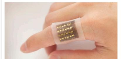
"A team of engineers at the University of California San Diego has developed an electronic patch that can monitor biomolecules in deep tissues, including hemoglobin. This gives medical professionals unprecedented access to crucial information that could help spot life-threatening conditions such as malignant tumors, organ dysfunction, cerebral or gut hemorrhages and more."
