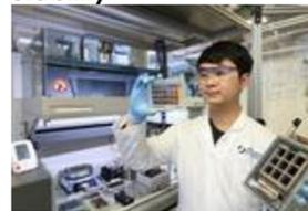
"In the current issue of the renowned journal Nature Energy, researchers from the Helmholtz Institute Erlangen-Nuremberg of the Forschungszentrum Jülich have presented a variant that stands out for its special stability. In tests at elevated temperature and illumination over 1450 hours of operation, the perovskite-based cell retained 99 percent of its initial efficiency."
