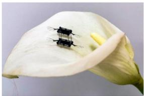
"Now, these researchers have pioneered a fabrication technique that enables them to build soft actuators that operate with 75 percent lower voltage than current versions while carrying 80 percent more payload. These soft actuators are like artificial muscles that rapidly flap the robot's wings."
