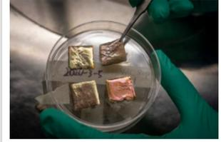
"Scientists have developed an all-season smart-roof coating that keeps homes warm during the winter and cool during the summer without consuming natural gas or electricity. Research findings reported in the journal Science point to a groundbreaking technology that outperforms commercial cool-roof systems in energy savings."
