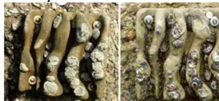
"the experimental tiles were constructed with crevices and grooved surfaces, based on the combination of ecological and engineering principles. The team attached the tiles with crevices of different depth to the vertical seawalls in Sham Shui Kok on Lantau Island and Lok On Pai in Tuen Mun in the western waters of Hong Kong for testing."
