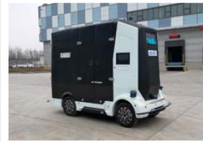
"Sensors include a main lidar, three auxiliary lidars, a stereo camera, four fisheye cameras, 16 sonars, redundant satellite navigation systems, an inertial measurement unit (IMU), and two wheel encoders."
