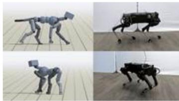
"Using a data set of motion capture data recorded from various sensors attached to a dog, the researchers taught a quadruped robot named Laikago several different movements that are hard to achieve through traditional hand-coded robotic controls."
