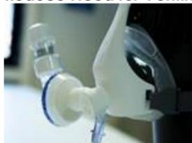
"The technology, designed with the help of pulmonologists, consists of a PEEP valve, a mask, and a filter. The patient wears a tightly fitted mask and the system needs only a source of oxygen to produce sufficient pressure to help a patient breathe."
