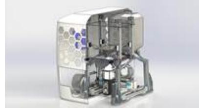
"The 3D printer developed at TU Graz melts metal powder using high-performance LED light sources and then processes it into components in additive manufacturing. The technology is similar to selective laser melting (SLM) and electron beam melting (EBM), in which metal powder is melted by means of a laser or electron beam and built up into a component layer by layer."
