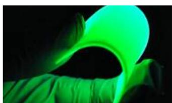
Florida State University researchers have developed a new material that could be used to make flexible X-ray detectors that are less harmful to the environment and cost less than existing technologies. Read more in [Nature](#).
