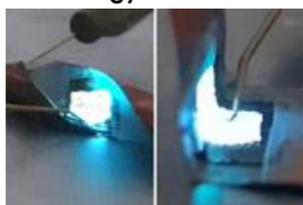
"University of Texas at Dallas researchers and their international colleagues have developed a method to create micro LEDs that can be folded, twisted, cut and stuck to different surfaces.."
