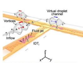
"The acoustofluidic process keeps the droplets contact-free above the substrate. With that advantage, the researchers guide one droplet after another along the same path without contamination."
