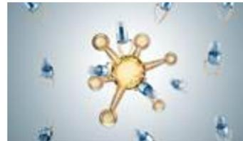
"The microrobot is layered with nickel and titanium oxide to ensure it can be magnetically manipulated and be biocompatible with the human body. Drugs can be loaded onto the porous, corkscrew-shaped scaffold and inside the needle."
