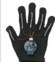
"The system includes a pair of gloves with thin, stretchable sensors that run the length of each of the five fingers. These sensors, made from electrically conducting yarns, pick up hand motions and finger placements that stand for individual letters, numbers, words and phrases."
