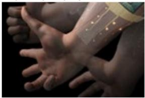
"UC Berkeley researchers have created a new device that combines wearable biosensors with artificial intelligence software to help recognize what hand gesture a person intends to make based on electrical signal patterns in the forearm."
