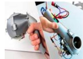
"The electronic tool is called Theia and it features gyroscope-based technology to pull the user in the correct direction. This is similar to how many virtual reality controllers work, but the direction of the pull would be decided using a mapping system that takes into consideration the ease and safety of a given path and other matters important to blind people."
