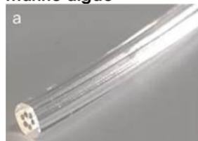
" An optical fiber made of agar has been produced at the University of Campinas (UNICAMP) in the state of São Paulo, Brazil. This device is edible, biocompatible and biodegradable. It can be used in vivo for body structure imaging, localized light delivery in phototherapy or optogenetics (e.g., stimulating neurons with light to study neural circuits in a living brain), and localized drug delivery."
