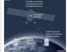
"The authors' meticulous optimization also involved cutting-edge signal acquisition, pointing and tracking systems and synchronization techniques for both the satellite and the ground stations."
