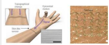
"The research team design this new measuring system that extracts signals corresponding to multiple finger motions by generating cracks in metal nanoparticle films using laser technology. The sensor patch was then attached to a user's wrist to detect the movement of the fingers."
