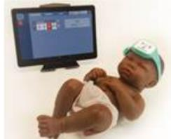
"The wearable wirelessly streams vital signs, such as respiration rate, to a phone or tablet computer, allowing healthcare staff to monitor newborns on the move or remotely."
