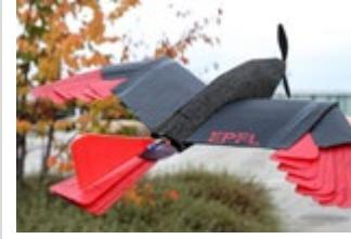
"EPFL engineers have developed a drone with a feathered wing and tail that give it unprecedented flight agility."
