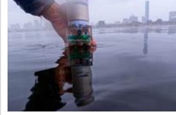
"MIT researchers built a battery-free pinpointing system dubbed Underwater Backscatter Localization (UBL). Rather than emitting its own acoustic signals, UBL reflects modulated signals from its environment. That provides researchers with positioning information, at net-zero energy."
