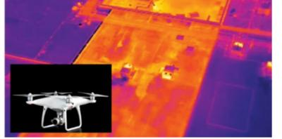
Hovering at 150 feet over the building, the drone can gather images and allow professionals to diagnose the status of the roof relatively quickly. These technological advances allow inspectors to gather a more comprehensive assessment compared to walking across the roof
