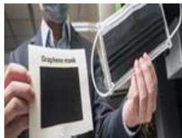
Researchers at the City University of Hong Kong have developed a face mask containing laser-induced graphene that can kill bacteria and has demonstrated potential in deactivating coronaviruses.
