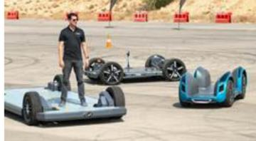
"As this new video from Israeli startup Ree demonstrates, the EV of tomorrow is basically just a giant skateboard. With tiny motors placed inside the wheels, the car can assume any form imaginable; any sort of seating or storage arrangement can be built right on top of this flat base."
