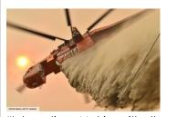
"Integrating Matrix with the Air Crane involves adding a digital fly-by-wire system, control actuators, and Sikorsky's perception software and sensor suite."
