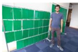
"That's the idea behind the CSAIL team's new system RFocus, a software-controlled 'smart surface' that uses more than 3,000 antennas to maximize the strength of the signal at the receiver. Tests showed that RFocus could improve the average signal strength by a factor of almost 10."
