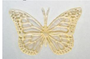
"Researchers at the University of Toronto Scarborough have, for the first time, turned waste cooking oil – from the deep fryers of a local McDonald's – into a high-resolution, biodegradable 3D printing resin."
