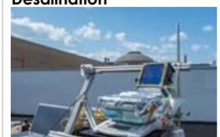
"A completely passive solar-powered desalination system developed by researchers at MIT and in China could provide more than 1.5 gallons of fresh drinking water per hour for every square meter of solar collecting area. Such systems could potentially serve off-grid arid coastal areas to provide an efficient, low-cost water source."
