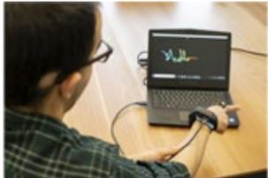
"Researchers at the University of Washington have created [AuroRing](#), a ring and wristband combination that can detect the precise location of someone's index finger and continuously track hand movements." Read more at [ACM](#).
