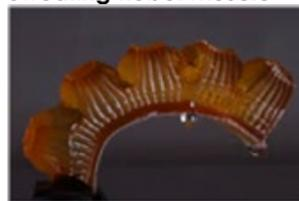
"Just when it seemed like robots couldn't get any cooler, Cornell researchers have created [a soft robot muscle](#) that can regulate its temperature through sweating ... The best part of this synthetic strategy is that the thermal regulatory performance is based in the material itself ... We did not need to have sensors or other components to control the sweating rate."
