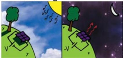
"A [thermoradiative cell](#) (right) generates electrical current as it radiates infrared light (heat) toward the extreme cold of deep space. UC Davis engineers propose that such cells could generate a significant amount of energy and help balance the power grid over the day-night cycle."
