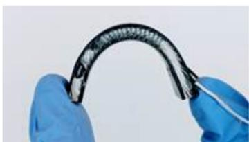
"North Carolina State University engineers have demonstrated a flexible device that harvests the heat energy from the human body to monitor health. The device surpasses all other flexible harvesters that use body heat as the sole energy source."
