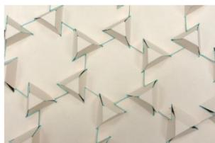
"Taking inspiration from both art forms, researchers [describe a new set of motifs](#) for creating lightweight, strong, and foldable structures using soft materials. These kirigami structures can support 14,000 times their weight and, because they don't require adhesives or fasteners, can easily be flattened and refolded."
