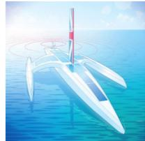
"The ship will cross the Atlantic to Plymouth, Mass., in 12 days instead of the 60 days of the 1620 voyage. It'll be made of aluminum and composite materials. And it will measure 15 meters and weigh 5 metric tons—half as long and 1/36 as heavy as the original wooden boat. Just as a spacefaring mission would, the new Mayflower will contain science bays for experiments to measure oceanographic, climate, and meteorological data."
