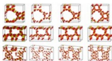
"Although progress has been made in creating small and simple molecules, complex materials such as crystalline porous materials have yet to be generated using any of the neural networks. Here, we have implemented a generative adversarial network that uses a training set of 31,713 known zeolites to produce 121 crystalline porous materials."
