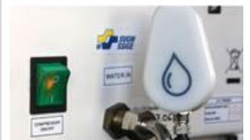
"Droople's smart meters record not just water flow rates and temperatures, but also peak usage times and total consumption—valuable data for facilities managers seeking to cut costs. The system consists of a series of smart flow meters installed at the point of use that collect data and send them through a low-power wide-area network (LoRaWAN) to a cloud-based software program."
