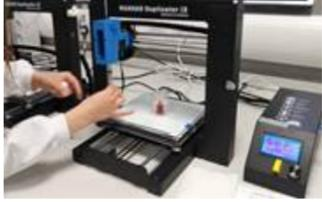
"A new way of 3D printing soft materials such as gels and collagens offers a major step forward in the manufacture of artificial medical implants."
