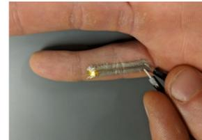
"The capability is possible thanks to two new advances. One is a new silver nanowire conductive ink. It can be printed at low temperatures and doesn't need additional processing."
