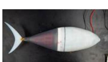
"The Tunabot is built from 3D-printed steel and resin, covered in a stretchy plastic skin. It mimics an adolescent tuna, but without any fins other than the tail. The robotic fish is 25.5 centimeters long, 4.9 centimeters thick and 6.8 centimeters high – this makes it a lot smaller than a real tuna. The skin of the robot tuna is around 1.5 millimeters thick."
