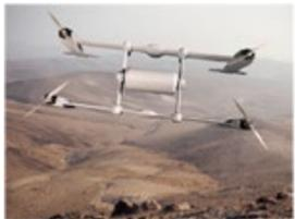
"The four-motor, vertical-lift electric UAV is one of the largest commercial cargo drone projects to reach the skies ... It weighs 300 pounds and can carry an additional 70 pounds of cargo, slung in an aerodynamic pod between its two wings."
