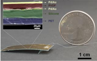
"The deceptively simple robot looks like a bent strip of paper, but it's able to move at 20 body lengths per second and survive being stomped on by a human wearing tennis shoes. Take that, cockroaches."
