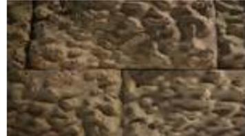
"The bricks, named 'Green Charcoal', contain more air pockets than a standard concrete block, making them up to 20 times more porous."
