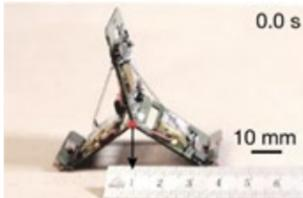
"Here we demonstrate an autonomous multi-locomotion insect-scale robot (millirobot) inspired by trap-jaw ants that addresses the design and scalability challenges of small-scale terrestrial robots."
