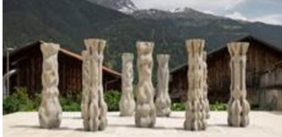
"A 3D printing process developed at ETH Zurich has been used to produce nine individually designed concrete columns. The fabrication process allows the production of concrete elements without the need for any formwork."
