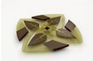
"An automated system developed by MIT researchers designs and 3-D prints complex robotic parts called actuators that are optimized according to an enormous number of specifications. In short, the system does automatically what is virtually impossible for humans to do by hand."
