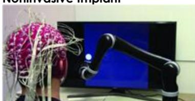
"Using a noninvasive brain-computer interface (BCI), the researchers have revealed the first-ever mind-controlled robotic arm that is able to track and follow a computer cursor."
