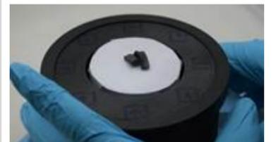
"Researchers have developed a new material which retains a given shape when it is put into a magnetic field. Unlike previous shape-memory materials, it consists of a polymer and droplets of a so-called magnetorheological fluid embedded in it."
