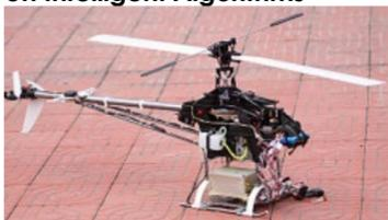
"This article designs an automatic flight control system for an unmanned aerial vehicle helicopter. The differential evolution intelligent algorithm is used for a state-space model identification; the differential evolution method has an advantage of choosing initial point randomly ..."
