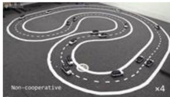
"The researchers, from the University of Cambridge, programmed a small fleet of miniature robotic cars to drive on a multi-lane track and observed how the traffic flow changed when one of the cars stopped."
