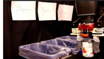
"The robot aims to reduce the reliance on human sorters and thus improve the viability of recycling operations. This is achieved through a novel approach of using special actuators that sort by material stiffness and conductivity."
