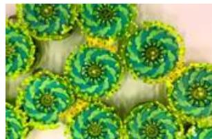
"Loosely connected disc-shaped 'particles' can push and pull one another, moving en masse to transport objects."
