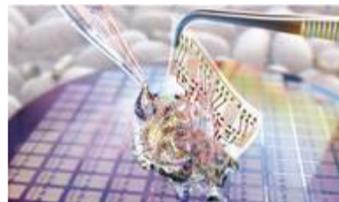
"Using photolithography instead of solvents, scientists in South Korea are now able to integrate silk fibroins with microelectronic components."
