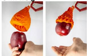
"As gas is pumped in and out of the gripper's airtight enclosure, the whole device opens and closes like a flower. This allows the device to pick up delicate objects without harming them, while still maintaining a strong enough grip to lift 100 times its own weight."
