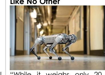
"While it weighs only 20 pounds, the cheetah has heavyweight skills like walking over uneven terrain, picking itself up after a fall or a swift kick and of course, its ability to pull off a 360-degree reverse flip from a standing position."
