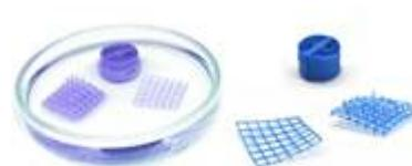
"A new, versatile plastic-composite sensor can detect tiny amounts of water. The 3d printable material, developed by a Spanish-Israeli team of scientists, is cheap, flexible and non-toxic and changes its colour from purple to blue in wet conditions."
