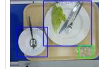
"Machine vision, AI used with robotics to create plate, cutlery and glassware sortation system for commercial kitchens."
