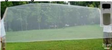
"A research team led by Prof. YU Shuhong from the University of Science and Technology of China (USTC) develops a simple solution based process to fabricate large-area Ag-nylon flexible transparent windows for high-efficiency PM2.5 capture."
