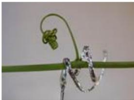
"Italian researchers have designed a soft robot that mimics the tendrils of a plant and has a movement system inspired by osmosis."
