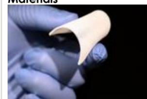
"Researchers have developed methods to 3D print piezoelectric materials that can be custom-designed to convert movement, impact and stress from any directions to electrical energy."
