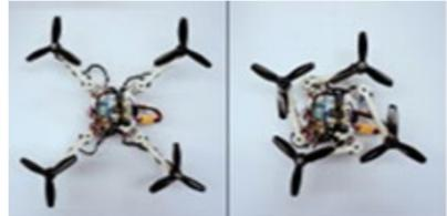
"We believe that a morphing quadrotor can tailor its shape to more dynamic tasks, like for example flying at high speed, where it can improve its performance by folding to change its aerodynamic properties. This would allow very fast flight in time-critical scenarios."
