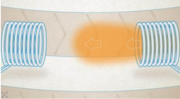
"If a commercially-viable magnetic field diode can be made, it could transform the capabilities of electrical components. It could, for example, enable wireless charging where energy only flows in one direction."
