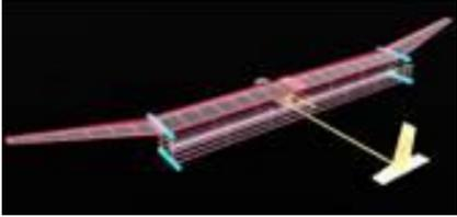
"Engineers at the Massachusetts University of Technology have built an ion-powered plane that flies without propellers or turbines, and requires no fossil fuel."
