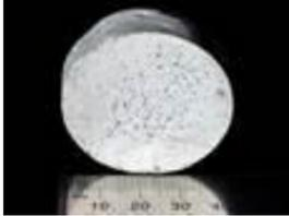
"A University of Melbourne researcher has discovered an organic, non-combustible and lightweight cladding core, a product that was previously thought to be impossible to create. Dr. Nguyen provided expert guidance in formulating a material that could withstand heat of 750 degrees Celsius."
