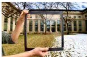
"MIT engineers have developed a heat-rejecting film that could be applied to a building's windows to reflect up to 70 percent of the sun's incoming heat. The film is able to remain highly transparent below 32 degrees Celsius, or 89 degrees Fahrenheit."
